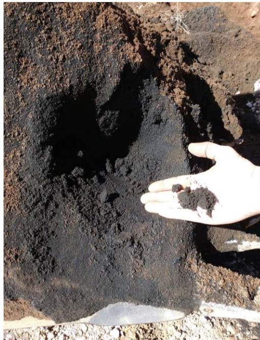
Figure 4: Non-homogeneous soil sample collected for testing
